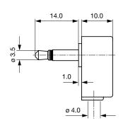
Cable diameter max. 4.0 mm
