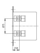
1) Line 2) Load 3) I/O connections torque 0.6...0.8 Nm
