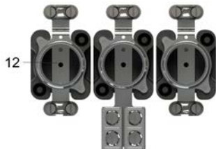
12. 63A- Fuse element with different connection variants
